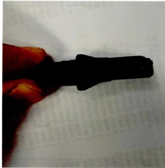
Figure 1 - Power cable yg terbakar
